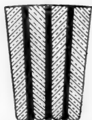
FIG. 134.—Sketch showing rounded edges of Commutator Segments.
